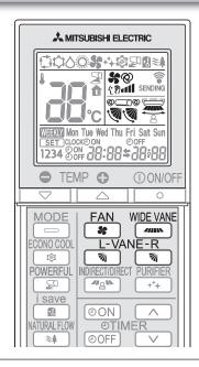
Press to select fan speed. Each press changes fan speed in the following order:
