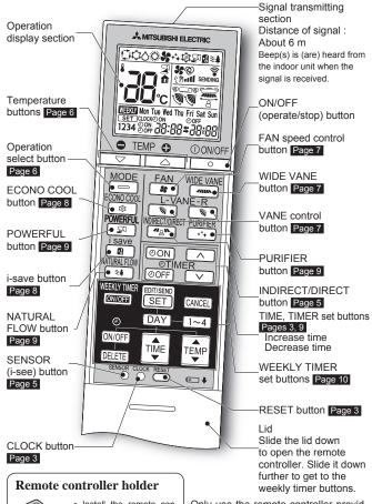
Install the remote controller holder in a place where the signal can be received by the indoor unit.
