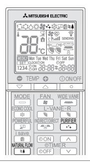
Press during COOL or FAN mode page 6 to start NATURAL FLOW operation.
